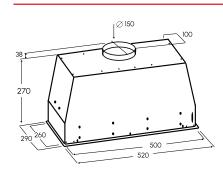
Cut-out Dimensions W502 x D270mm
